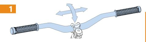
Align the handlebar centrally and adjust the handlebar's tilt according to personal preferences. Adjust the brake and gear levers to match the handlebar's angle.
